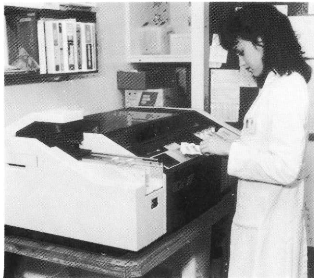
Lab. Assistant Pania Tetau loads blood samples into the ACA SX analyser. Fully automatic operation allows a 24 hour service for a wide range of Biochemical tests.
