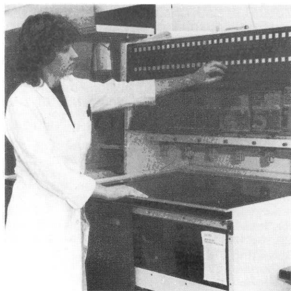
Medical Technician, Mrs. Karen Fitzgerald using the Pathology Department Automatic Chemistry Analyser (ACA) which performs a wide variety of blood serum tests.
