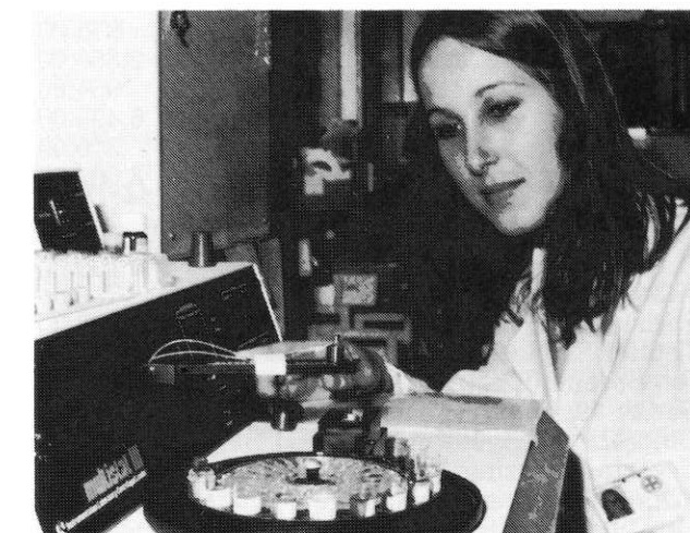
Medical Technician Julie Heald checks the operation of a Multistat Analyser used for chemical testing of blood serum.
